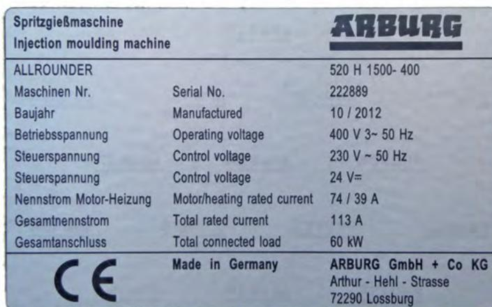
The image shows a metal identification plate for an ARBURG injection moulding machine. The plate is rectangular with a blue background and white text. At the top left, it says 'Spritzgießmaschine' and 'Injection moulding machine'. At the top right, the ARBURG logo is displayed. Below this, there is a table of technical specifications. At the bottom left is the CE mark, and at the bottom right is the manufacturer's name and address.
