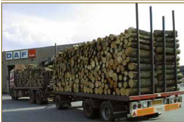
Fig. 69. Timber stacked transversely is not recommended!
