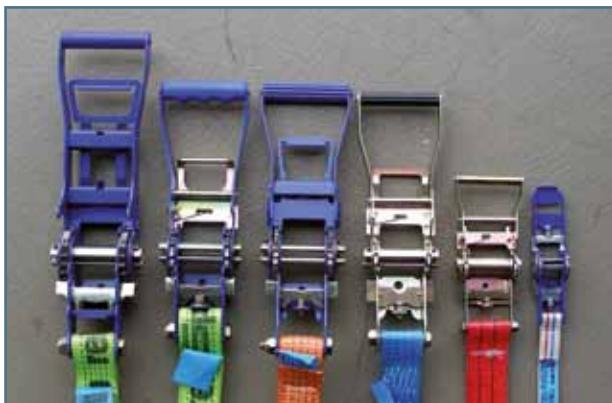
Fig. 37. Different types of ratchets
