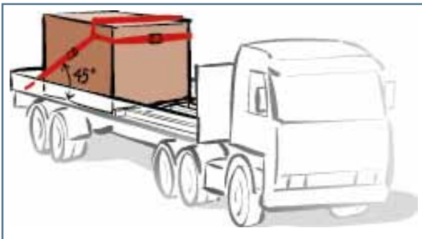
Fig. 26. Example a spring lashing preventing forward movement
