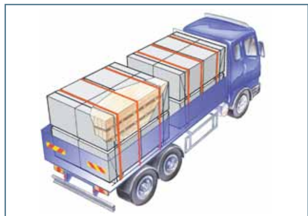
Fig. 51. Secured full load of sawn timber
