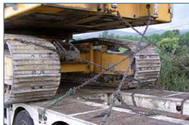
Fig. 39. Excavator diagonally lashed with chains
